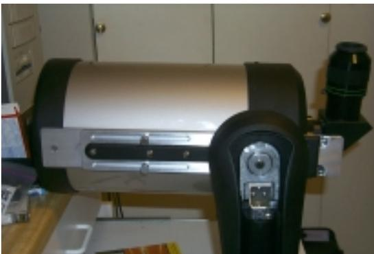
Now install the OTA to the arm. Also install your diagonal and your heaviest Eye Piece. Now slide the OTA back and forth to find the balance point. On mine with a CI 1¼" Diagonal and a 40Mmm Eye Piece, the balance point is ¼" forward.
