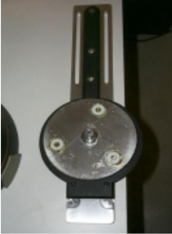
Install the Clutch disk on the OTA arm. After that install the Driven gear to the arm.
