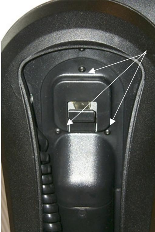
After removing the hand controller, you will see the Dec nut cover held on by three allen screws.
